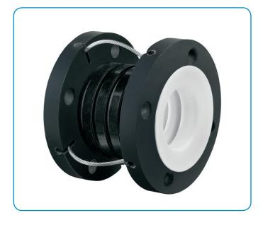
These flexible PTFE connectors and tremor barriers are designed to compensate for misalignment, absorb expansion and contraction, and isolate the vibration and shock that could damage a tank. Their low spring rate protects stress-sensitive connections. Can be installed directly to the dome of the tank to overcome piping misalignment
