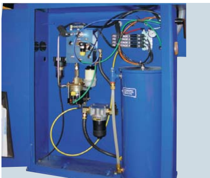
Exclusive integrated hydraulic circuit technology automatically compensates for varying pressures and temperatures. The enclosed steel cabinet and leak-free design minimize maintenance.
