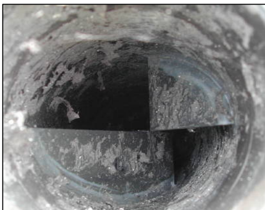
Statiflo Sludge Blender after 90 hours
